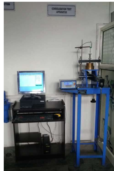
Digital Consolidation Test Apparatus
