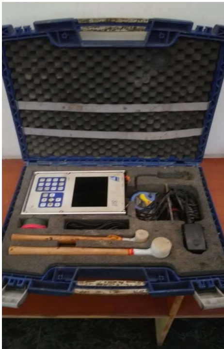
Pile Integrity Test Machine
